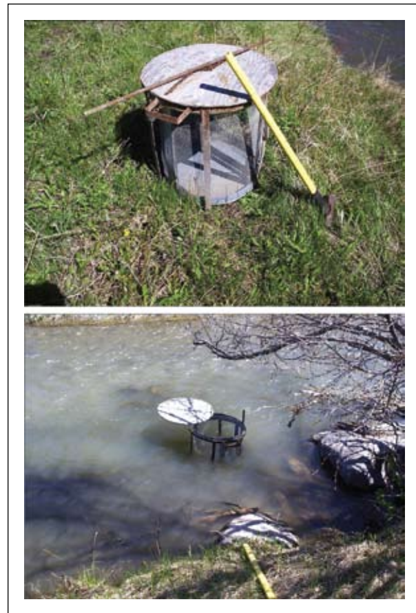
Figure 12. Sentinel cages are used in field experiments to assess M. cerebralis infection risks under natural conditions. The cages are anchored in the stream with test subject fish contained inside.
